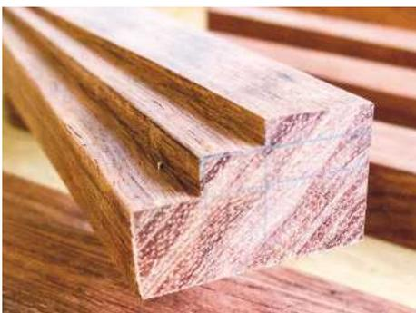
**Bubinga's interlocked grain made hand planing the tapers a real chore; you can see where a custom cutter would've saved a lot of blood and sweat**
